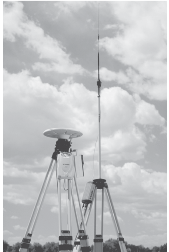
FIGURE 1-3 Zepher™ geodetic GPS antenna, with a 5700 GPS receiver and radio communications equipment. Zepher antennas are said to have accuracy potentials similar to those of choke ring antennas—at lower costs
