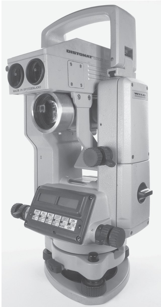
FIGURE 1-5 Early model of an electronic theodolite with interfaced Distomat EDM (mounted on the telescope).
